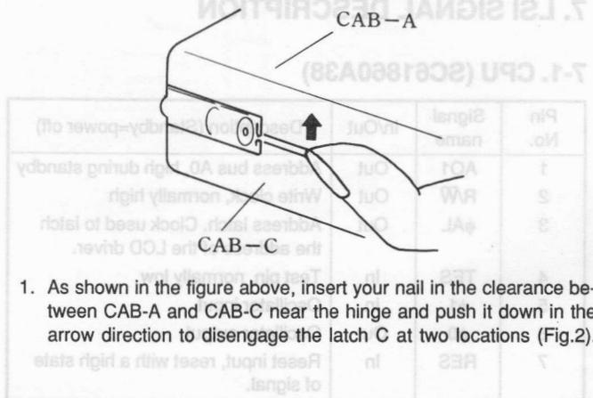
1. As shown in the figure above, insert your nail in the clearance between CAB-A and CAB-C near the hinge and push it down in the arrow direction to disengage the latch C at two locations (Fig.2).
