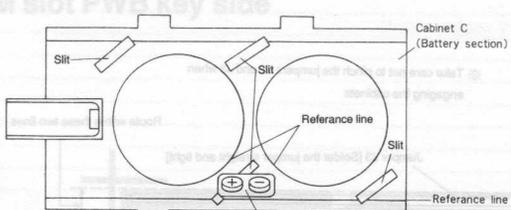
※ When attaching the label, be careful not to fall into the slit shown in the figure.
