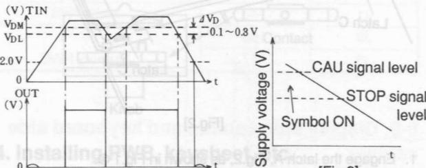
Action of the voltage detect IC [Fig.2]
