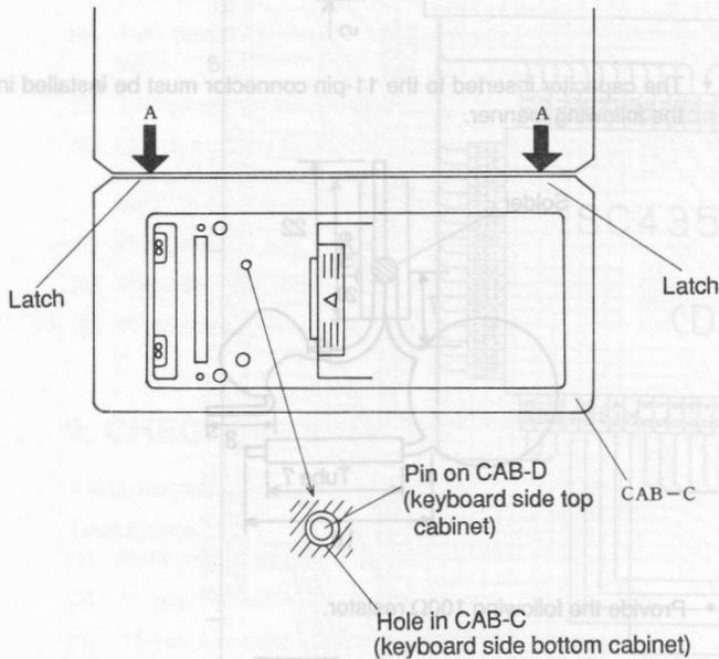
\*The pin must be properly and firmly engaged in the hole.
