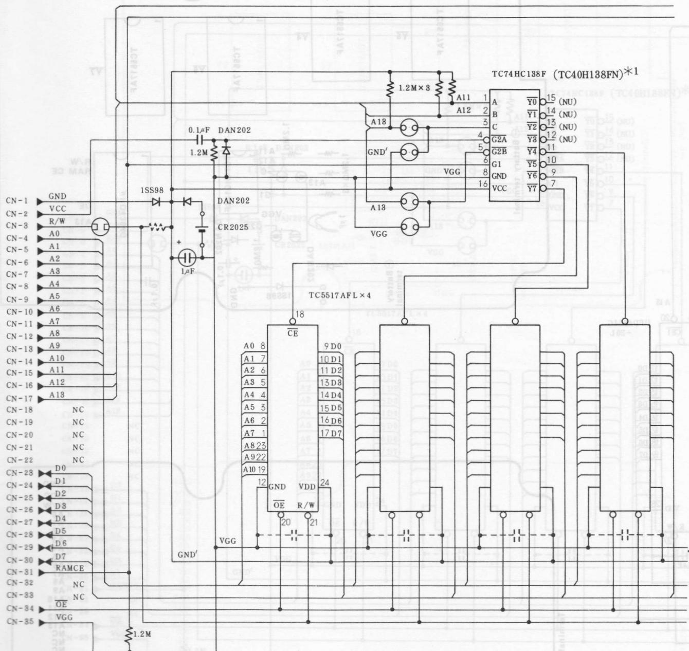
\*1: On account of parts procurement situation, the TC40H138FN was used as a substitution of the TC74HC138F for some of CE-201M and CE-202M in earlier productions. When the TC40H-138FN is in failure, either the TC40H138FN or TC74HC138F can be used as a replacement. But when the TC74HC138F is in use, it has to be replaced by the TC74HC138F, not the TC-40H138FN which may impede proper operation due to variation in access time by the RAM chip used.
