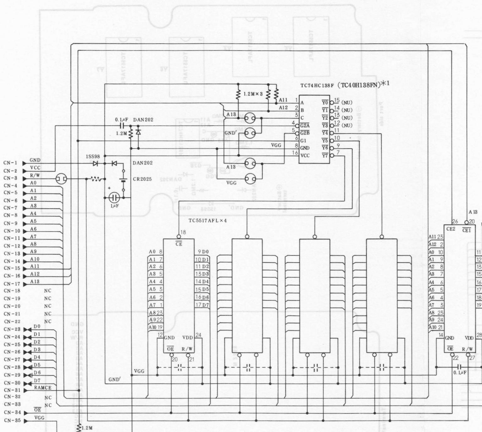
\*1: On account of parts procurement situation, the TC40H138FN was used as a substitution of the TC74HC138F for some of CE-201M and CE-202M in earlier productions. When the TC40H-138FN is in failure, either the TC40H138FN or TC74HC138F can be used as a replacement. But when the TC74HC138F is in use, it has to be replaced by the TC74HC138F, not the TC-40H138FN which may impede proper operation due to variation in access time by the RAM chip used.
