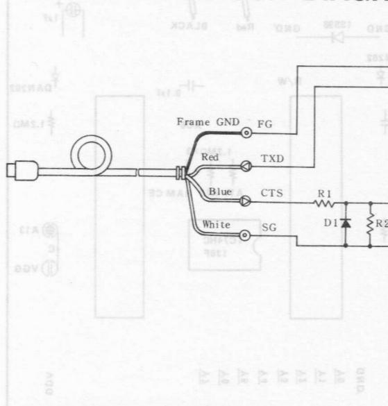
15-pin connector pin description (to PC-1350)
