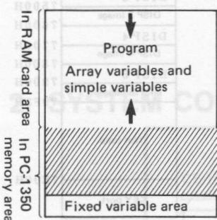
Execution of the MEM "C" command makes variables held on the RAM card, so that they remain on the RAM card even after it has been removed from the PC-1350.
