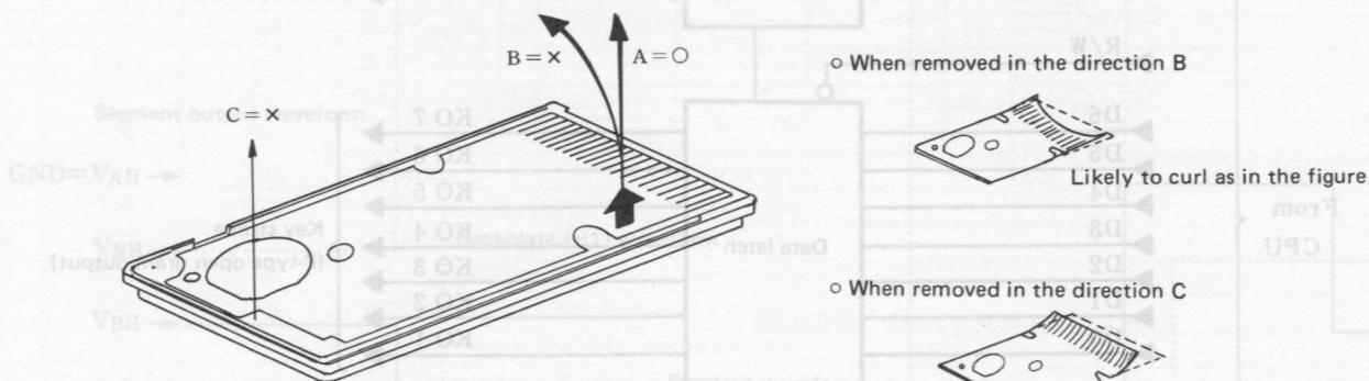
Bonding the curled terminals on the cabinet may result in terminal contact failure. Make the deformed board unit corrected so that a slight degree of curl should appear in the opposite direction, and use the fresh tape to bonding the board on the cabinet.
