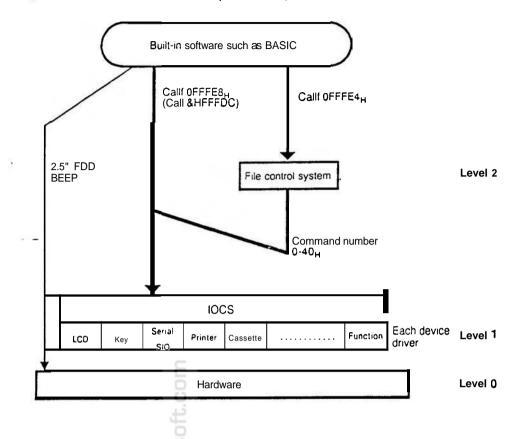
When creating program with this pocket computer, it is recommended to use level "0" (direct operation of hardware) only when you have to perform quick processing to correspond to succeeding device. (Actually, it is better not to use level 0.)
