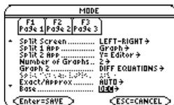
**Note:** To display different graphs in both parts of a split screen, you must use the **2-graph** mode.
