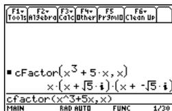
Calculator screen showing the complex factorization of  $x^3 + 5x$  with respect to  $x$ . The input is  $\text{cfactor}(x^3 + 5x, x)$ . The output is  $x \cdot (x + \sqrt{5} \cdot i) \cdot (x - \sqrt{5} \cdot i)$ . The status bar at the bottom shows MAIN, RAD AUTO, FUNC, and 1/30.
