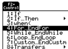
When you select a loop, the loop command and its corresponding **End** command are inserted at the cursor location.
