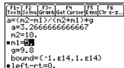
**Note:** To stop (break) a calculation, press **[ON]**. The unknown variable shows the value being tested when the break occurred.
