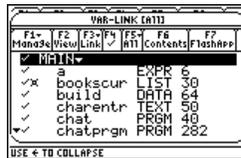
4. On the *receiving* unit, press [2nd] [VAR-LINK] to display the VAR-LINK screen. (The sending unit remains on the VAR-LINK screen.)
